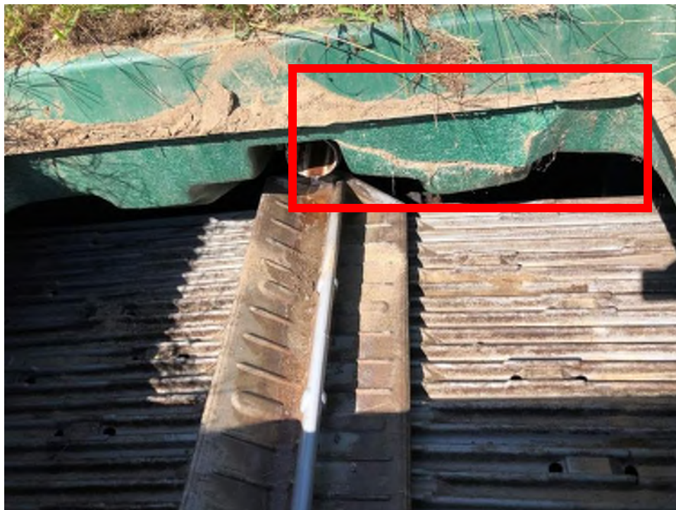
Figure 23: Significant damage to Ecoflo #5. 40-50 cm crack.
