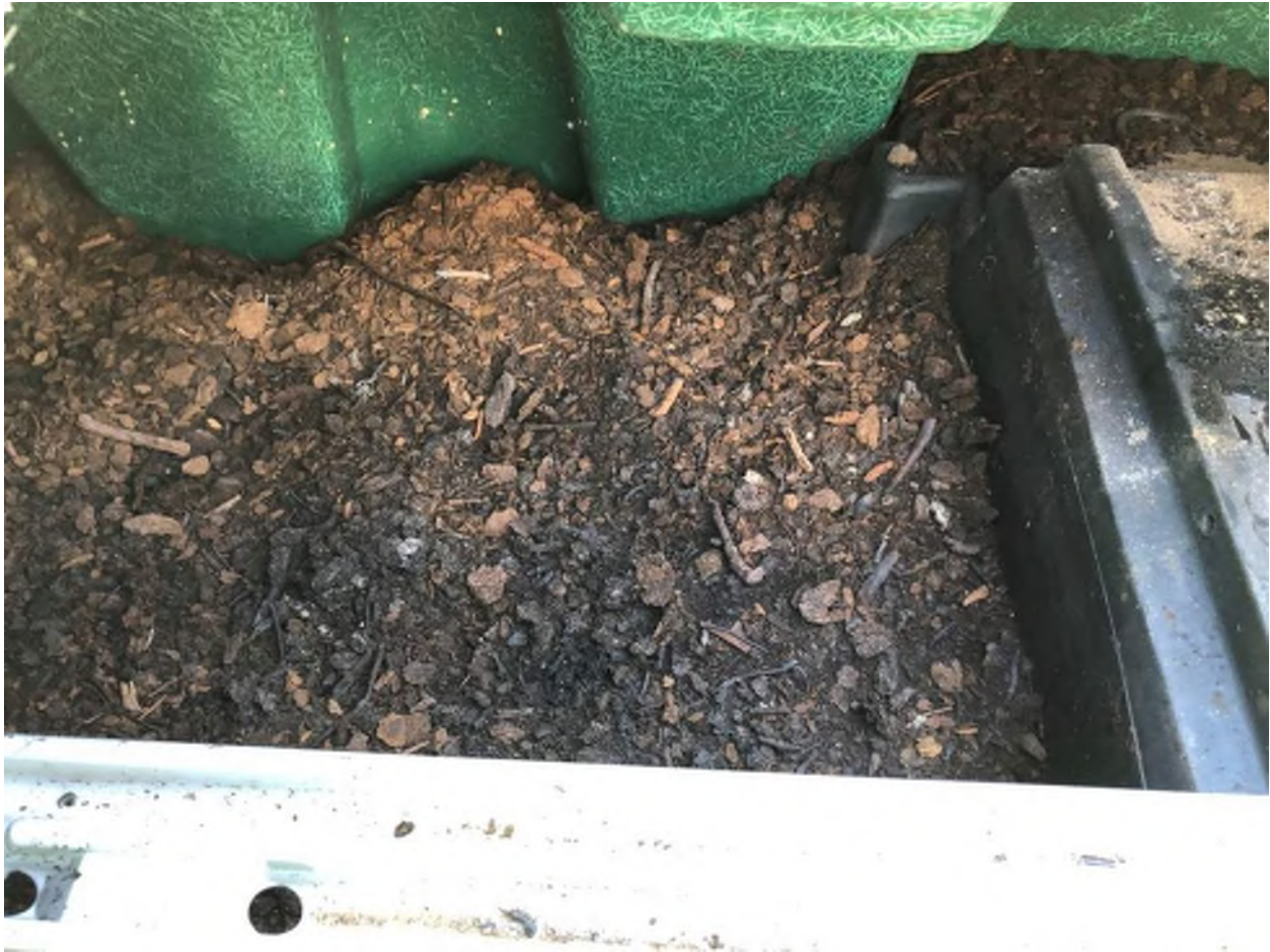
Figure 27: Typical state of the peat filter media in the treatment units observed.
