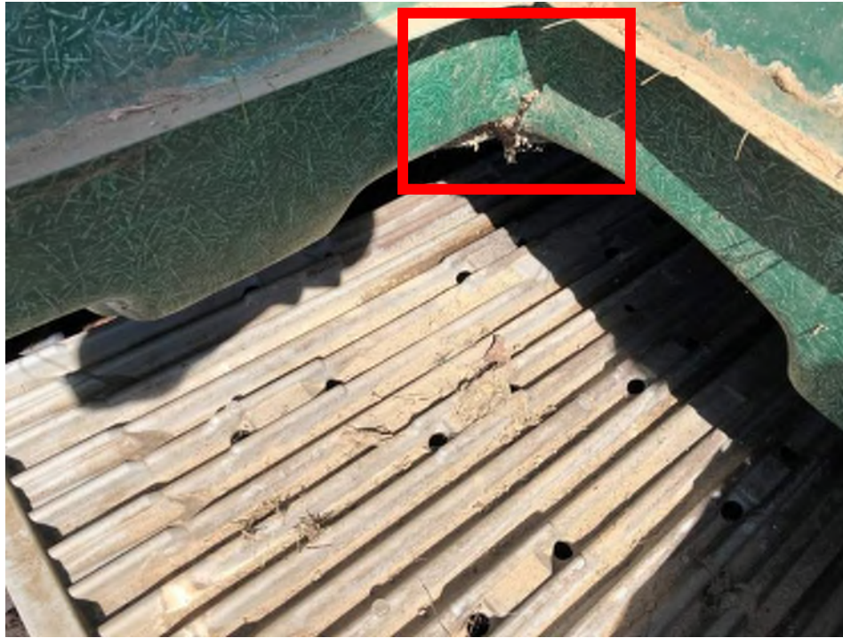
Figure 25: Small 15 cm crack in fibreglass shell of Ecoflo #7.
