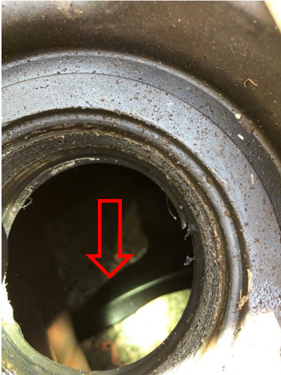
Figure 24: Piece of fractured plastic observed through central access port of Ecoflo #6.
