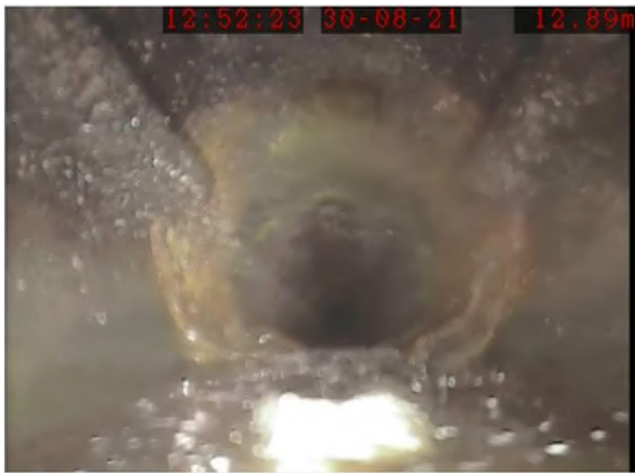
Figure 8: Internal view of the sewer as the sewer camera began to advance beneath the floor slab.
